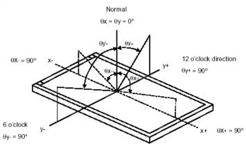
Note 7: Measured at the center area of the panel when all the input terminals of LCD panel are electrically opened. Note8: The method of optical measurement:
